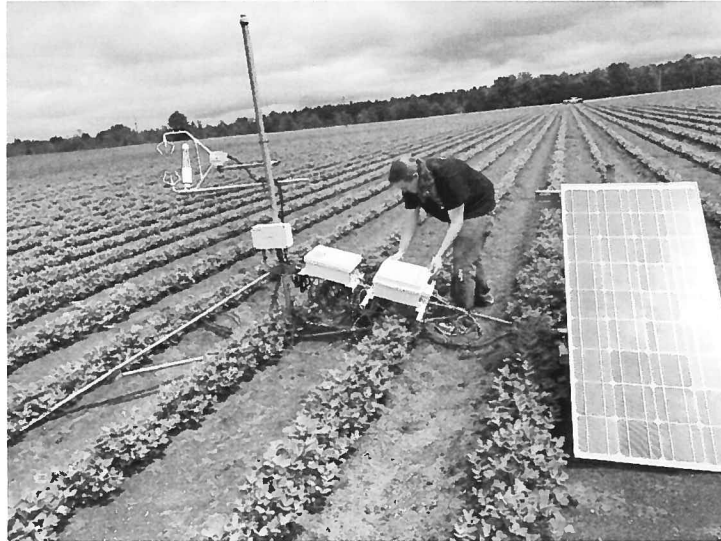
Figure 1. Eddy-covariance system in the peanut field
