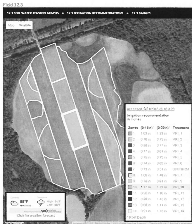
Figure 2. Dynamically developed irrigation scheduling recommendations for each IMZ. Clicking on either the zone or the recommendation will highlight both. In the figure, zone 10 is highlighted. The recommendations are to bring the soil profile to within 75% of field capacity.
