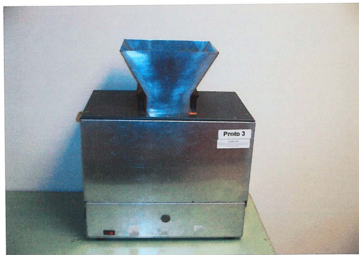
Figure 3: Portable Prototype Microwave Moisture Sensor (shown with detachable funnel)
