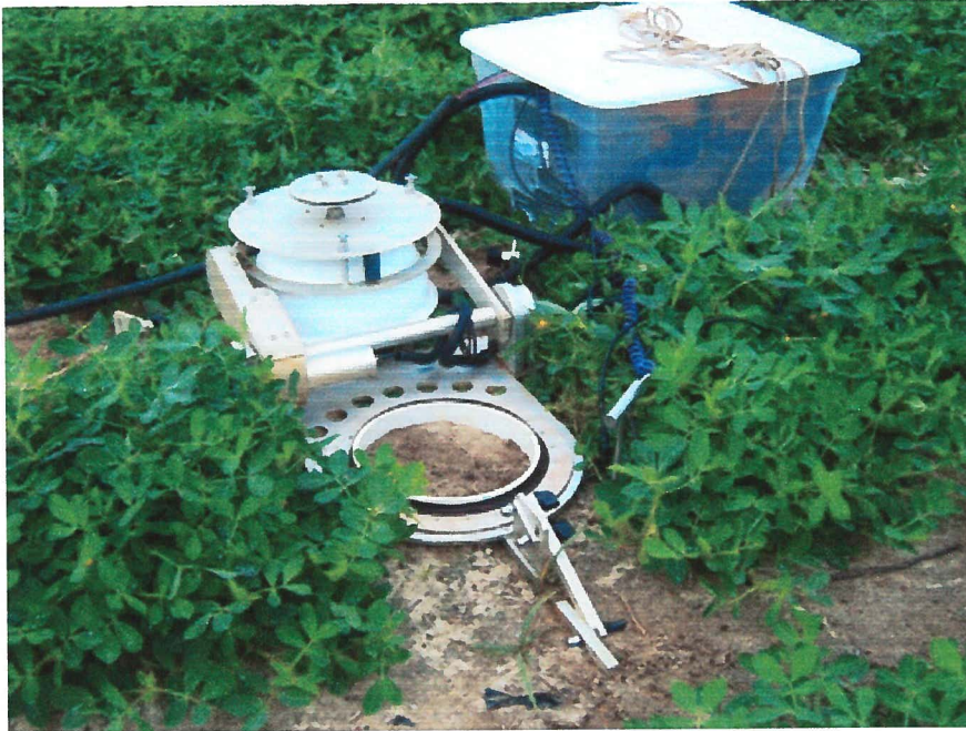
Figure 2. A long-term low-frequency automated soil chamber (Li-8100-101, Li-Cor, Inc., Lincoln, NE).
