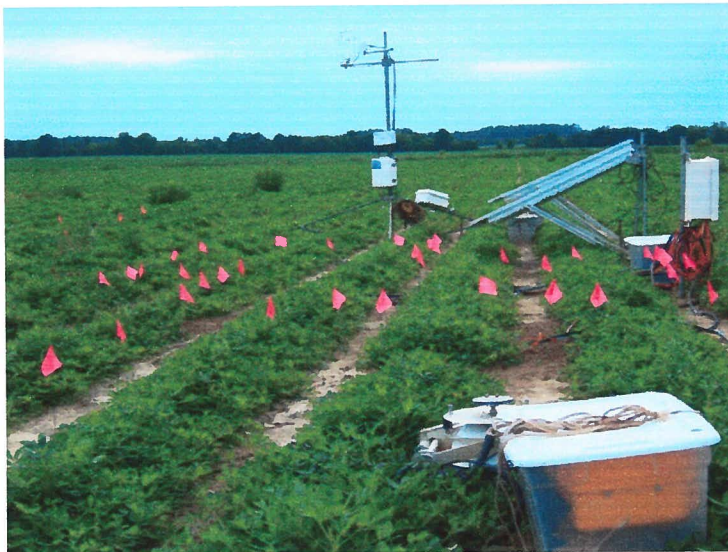
Figure 1. Sonic anemometer, fast infrared gas analyzer setup for measuring CO 2 exchange and solar panels setup for power support to all instruments.
