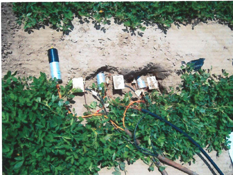
Figure 3. High-frequency soil CO 2 gradient method (GMP343 soil CO 2 probes, Vaisala Inc., Vantaa, Finland).
